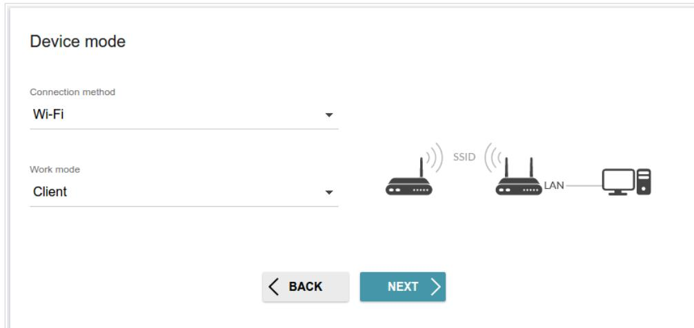
Figure 39. Selecting an operation mode. The **Client** mode.
